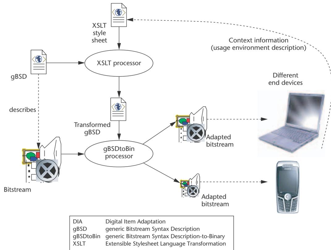
**Figure 1. Multimedia publishing using MPEG-21 DIA according to different usage contexts.**
